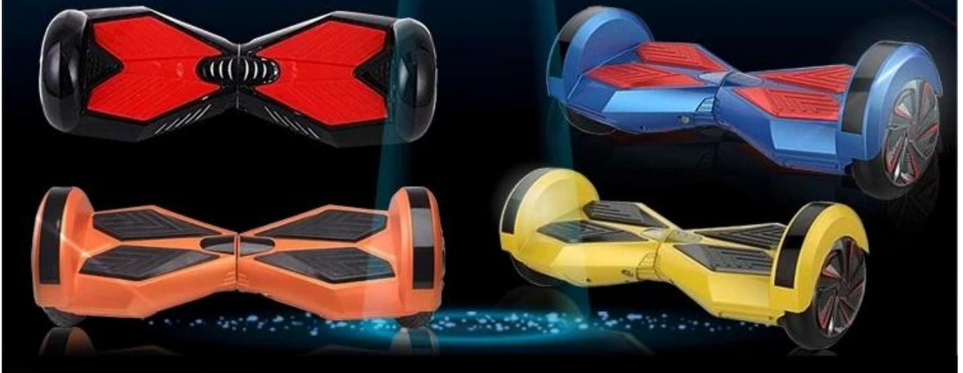
*It uses space attitude control algorithm, fuzzy algorithm, the gyroscope system and the inverted pendulum system, achieve forward, acceleration, deceleration, brake and vehicle operation, about the direction of the balance depends on the body twist.*
