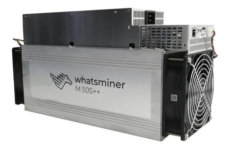
Miner is based on 8nm Samsung Asic technology.
